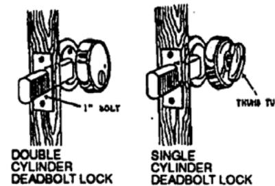
A single cylinder deadbolt lock should be mounted on a solid wood core door when there is no breakable glass within 40 inches of the interior locking mechanism. The single cylinder deadbolt lock has a thumb turn piece on the inside.
